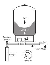
The amount of water delivered between pump cycles is called drawdown. The larger the well tank, the greater the drawdown capacity, the less the pump needs to run. This saves energy and money, and extends pump life. Larger tank sizes also increase the water storage volume to provide more consistent water pressure.
