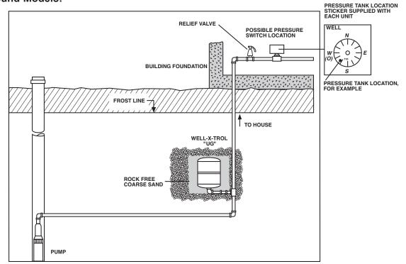
All Well-X-Trol Underground Tanks are designed for direct burial and must be installed in the vertical position **only**. To eliminate danger of freezing, tank should be buried below the frost line.
